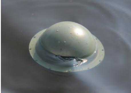
Riverine Drifter deployed in Pearl River, Mississippi
