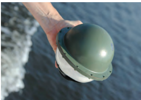
Conceptual design of Riverine Drifter dispenser pod for Tier 2 UAV
