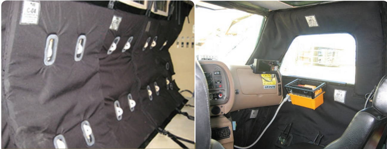
Spall Liner shown installed inside a land vehicle
